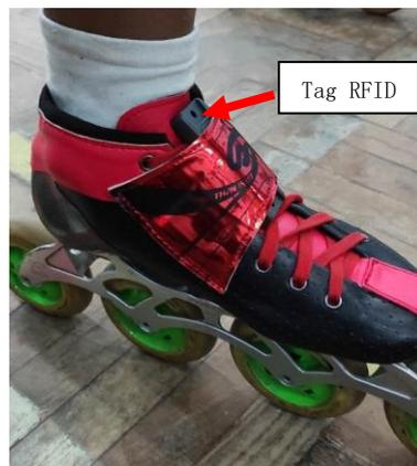
Figure 21. RFID Tag On Roller Skates
