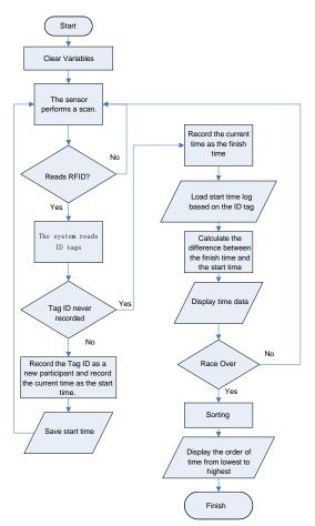
Figure 3. Planned system workflow
