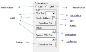
Figure 18. Serial connection module display
