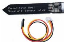
Gambar 1. Sensor *Moisture Soil*
