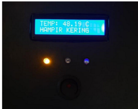
Gambar 5. Indikator Deteksi Suhu Hampir Kering
