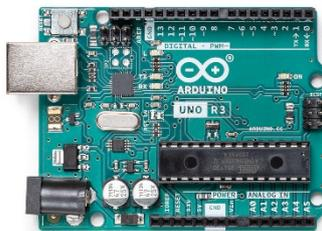
Gambar 1. Board Arduino UNO R3
