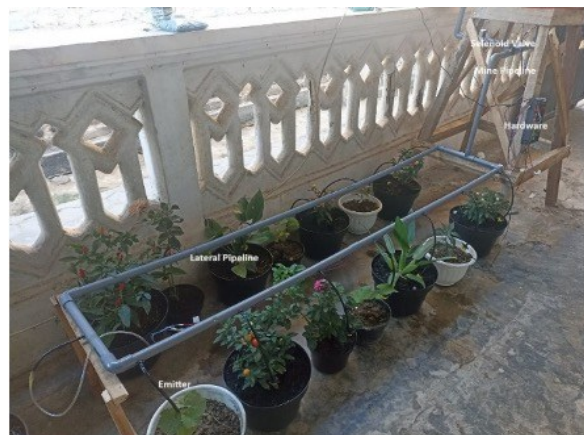
Fig 9. Model of Drip Irrigation System
