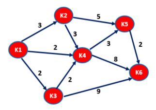
Figure 2. ILLUSTRATION OF DIJKSTRA'S ALGORITHM
