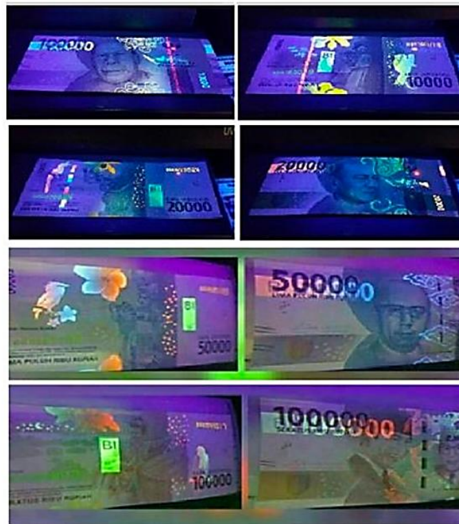
Figure 1. Appearance Of Rupiah Currency When Exposed To Ultraviolet Light
