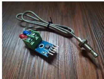
Gambar 4. MAX6675 & Thermocouple Type K
