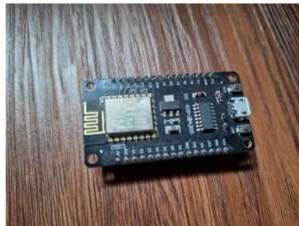
Gambar 1. NodeMcu ESP8266
