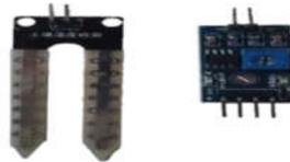
Gambar 6. Sensor Soil Moisture YL 100
