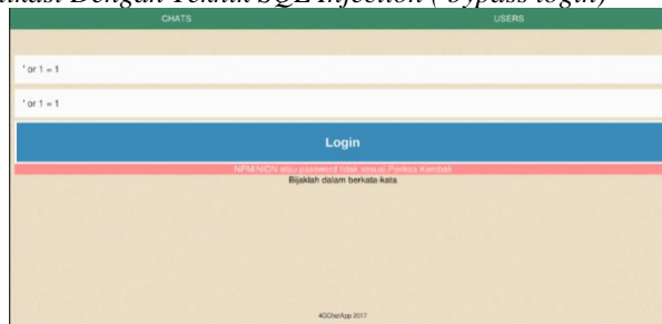
Gambar 10. Pengujian SQL Injection ( bypass login)
