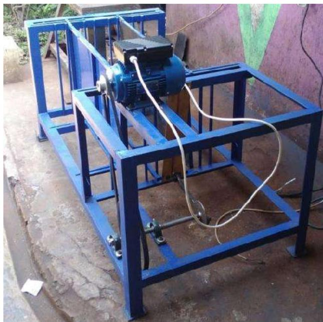
Gambar 3. Mesin Poles Biting Bambu
