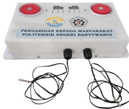
Gambar 7. System controlling suhu berbasis IoT
