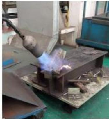
Gambar 4. *Normalizing heat treatment part cutter*
