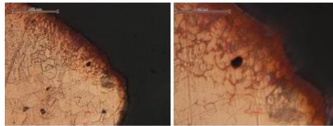
Figure 3.7 Results of inspection of the macro and micro structures of copper wire experimental results of short circuit treatment at 800% ACC (144 Ampere).
