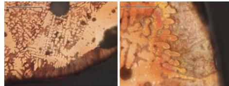
Figure 3.8 Results of examining the macro and micro structures of copper wire from the overload treatment experiment, current 800% ACC (144 Ampere).
