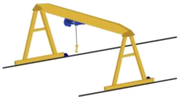
Gambar 1. Single Girder Gantry Crane
