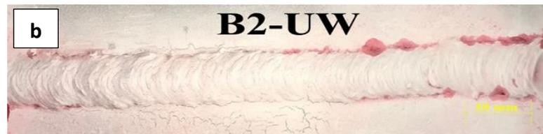
**Figure 3.** Samples of test results with liquid penetrant
