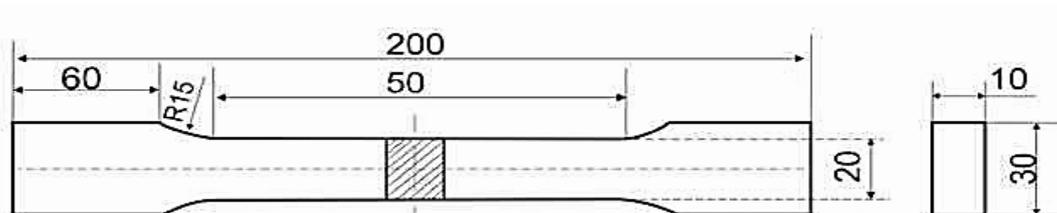
**Figure 2.** Tensile test sample dimensions
