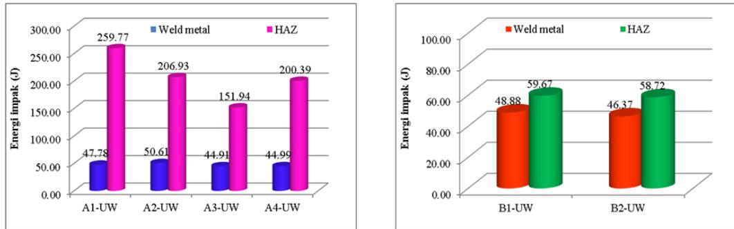
**Figure 7.** Comparison of impact toughness values of WM and HAZ steel AH-36 with Electrode (a) E6013 Modified Magnesium and (b) Broco E70XX.
