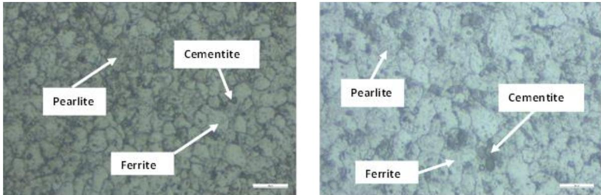
**Figure 5.** Weld metal microstructure (a) B1-UW heat input 1.5 kJ/mm 500x magnification, (b) B2-UW heat input 2.5 kJ/mm 500x magnification
