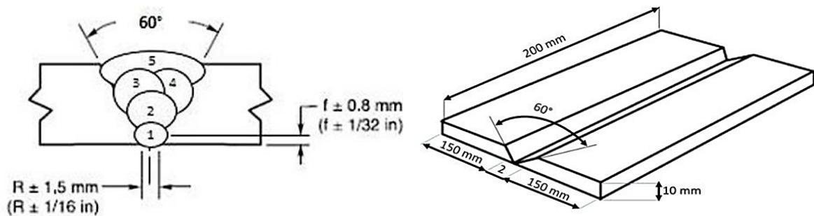
**Figure 1.** Preparation Welding of marine steel plate AH-36:
