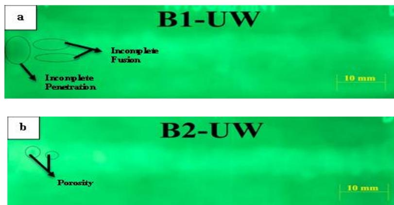
**Figure 4.** Results of testing with gamma-ray radiography:
