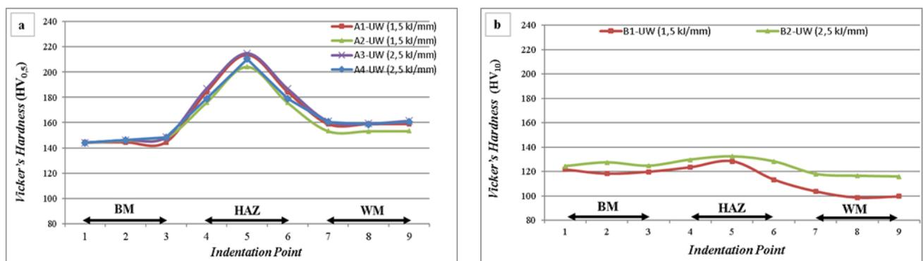
Figure 6. The results of the Vickers hardness test at a depth of 2 mm with electrodes (a) electrodes E6013 modified Mg (b) Broco E70XX
